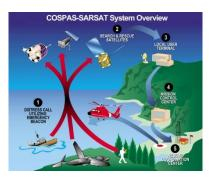
an earth station called the Local User Terminal (LUT), which may be within the view of the satellite, as well as being stored for later transmission to other LUTs.
